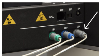
Figure 3. Connecting the Penis Safety Probe to CoreTherm® SE.
