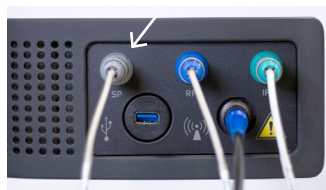
Figure 4. Connecting the Penis Safety Probe to CoreTherm® Eagle.
