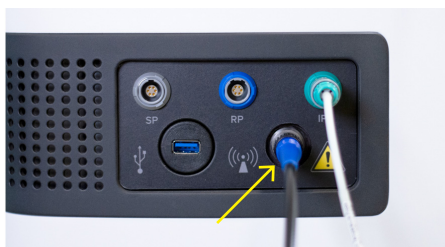
Figure 4. Connecting the Microwave Antenna to CoreTherm® Eagle.
