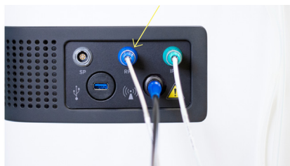
Figure 3. Connecting the Rectal Temperature Probe to CoreTherm® Eagle.
