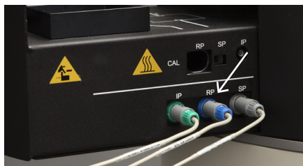
Figure 4. Connecting the Rectal Temperature Probe to CoreTherm® / SE.
